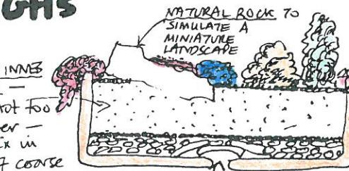
DRAINAGE HOLE It is essential to keep the trough well drained: cover hole with a few bits of old crock. Then a good layer of coarse gravel & add a fine layer of gravel to "steep out" soil being washed down
